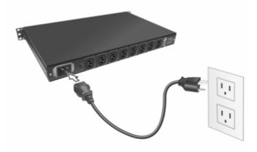
After power connected. You may see the 7-Segment LED display some error messages. If it shows "**E01**", please refer to section 2.6 to connect IP Power Manager 8000 to your LAN or WAN. If it shows "**E16**", that is mean the power phase of connected power outlet is reverse. Please try to make the power phase correct. Or you can refer to section 5.2.2 to disable Input Phase Detection on IP Power Manager temporally. For other error message, please refer to Appendix A Error Code for details.
